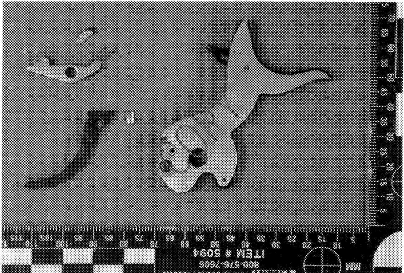
Item 2 cylinder stop/bolt (top left) and trigger sear (bottom left) are fractured, hammer (right) is intact
