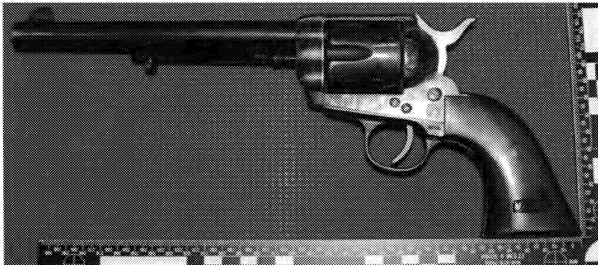
Item 2 is a .45 Colt (.45 Long Colt) caliber F.lli Pietta revolver, Model 1873 SA (Californian)
